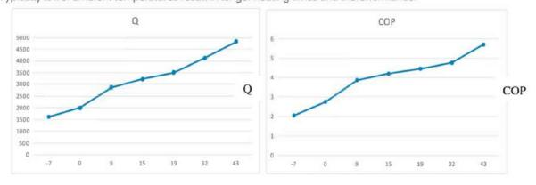
Changes in ambient temperature and heating capacity
